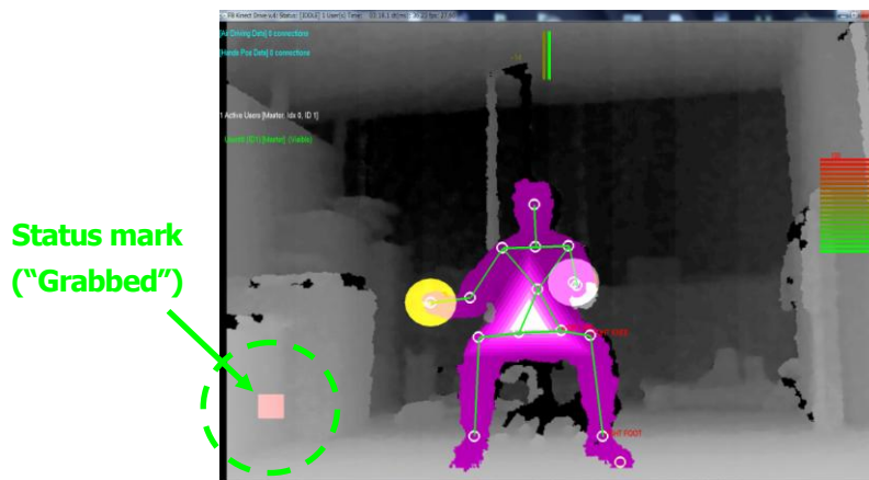
Figure 12: Air Driving. The user grabs the virtual gear lever (square-shaped indicator in the bottom left side of the window)
